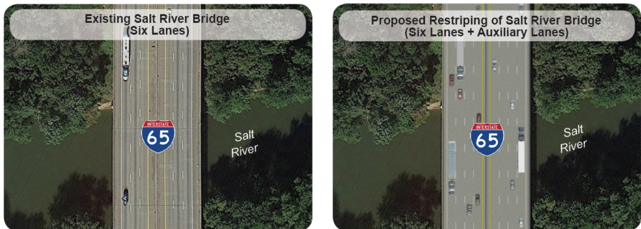
Figure ES-2: Restripe Salt River Bridge (both directions) to Extend Auxiliary Lanes on I-65 between the KY 480 (Exit 116) and KY 44 (Exit 117) Ramps
